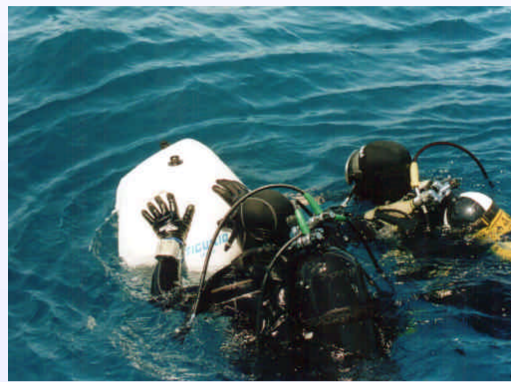
Fig.4- Sampling boxes retrieving with lifting balloon
