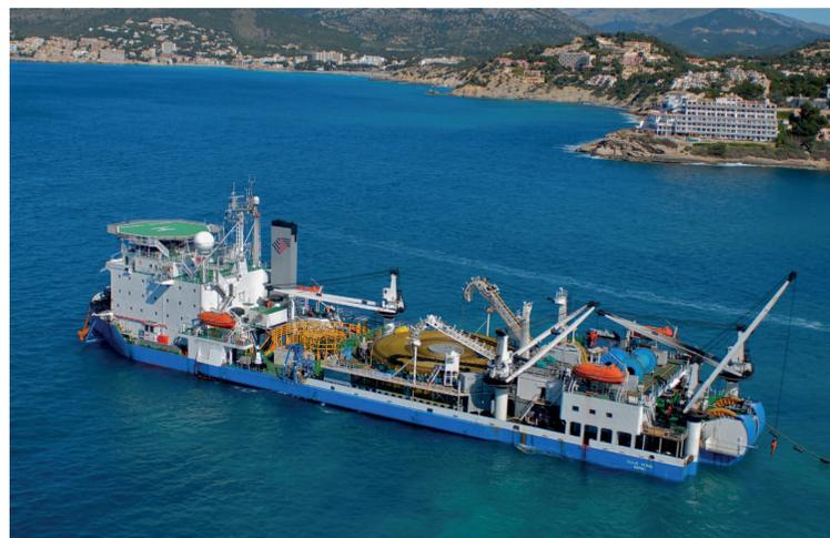
Cable-laying vessel (Source: Prysmian Group)
