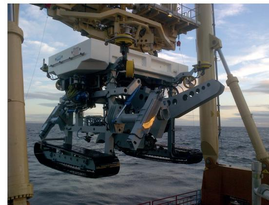
*Cable trenching ROV prior to deployment
